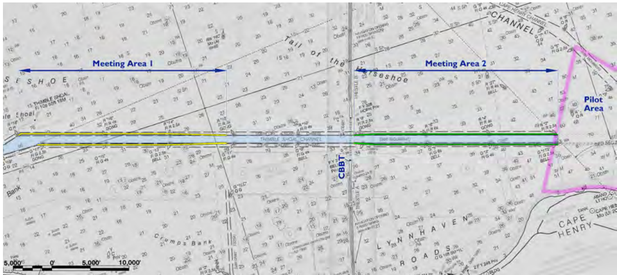
Figure 3. Meeting Areas at the Thimble Shoal. The previous Norfolk Harbor Navigation Improvements GRR/EA Recommended Plan (Preferred Alternative) only included the Meeting Area 2. With the Norfolk Harbor Validation Study/Supplemental Environmental Assessment, Meeting Area 1 is being proposed as an additional meeting area.
