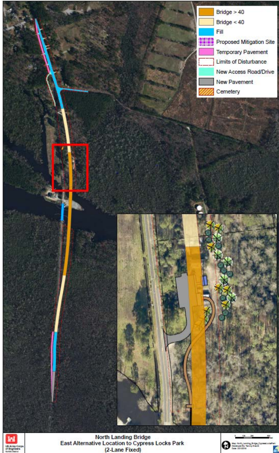
Figure 7-7. East Alignment Fixed Bridge crossing the proposed park. (NOTE: Park building configuration drawing is conceptual).
