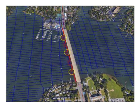
Figure 2-2-2. The Proposed Small-Barrier Configuration with 5 Floodgates (yellow circles designate floodgates that will be closed for scenario simulation of S04).
