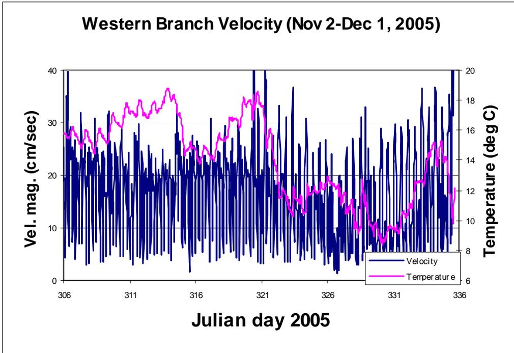
Figure IV.10. Western Branch velocity and temperature.
