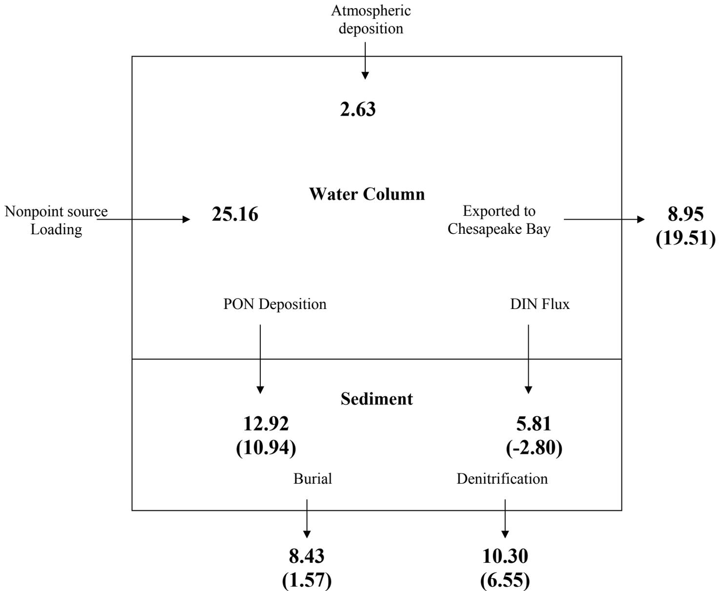
Figure VII.2. Annual Total Nitrogen budget (mg N m<sup>-2</sup> d<sup>-1</sup>) for Lynnhaven River (Values in parentheses indicate results without BMA)
