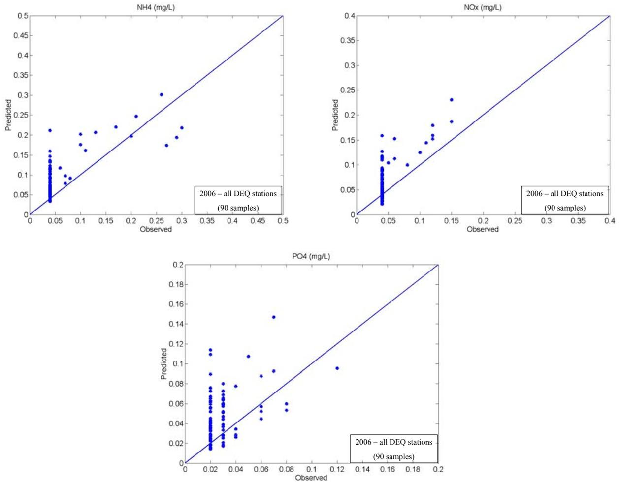
Figure V.41. Plots of 1:1 predicted vs. observed NH<sub>4</sub>, NO<sub>x</sub>, and DIP.
