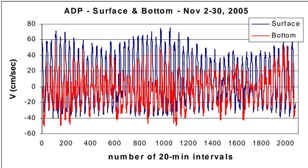
Figure IV.6. ADP velocity outside Inlet.
