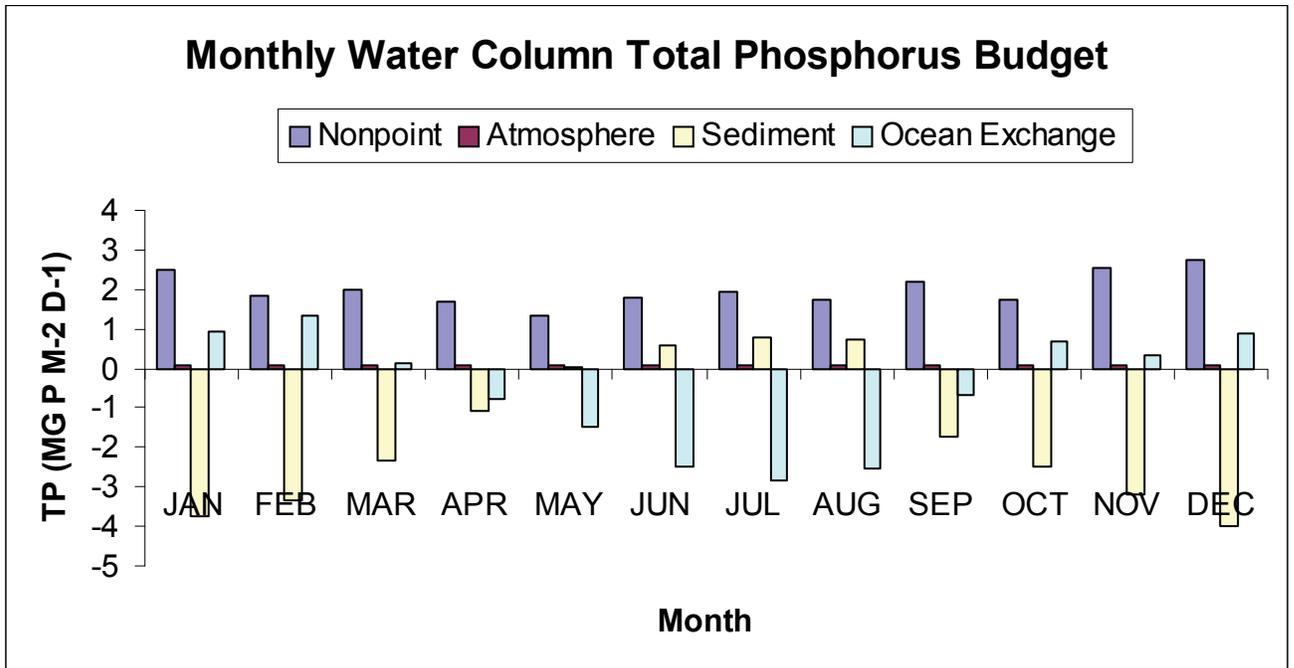
Figure VII.6. Monthly Total Nitrogen budget ( $\text{mg N m}^{-2} \text{d}^{-1}$ ) and Total Phosphorus budget ( $\text{mg P m}^{-2} \text{d}^{-1}$ ) in the water column for Lynnhaven River (positive means entering the water column, and negative means leaving the water column)
