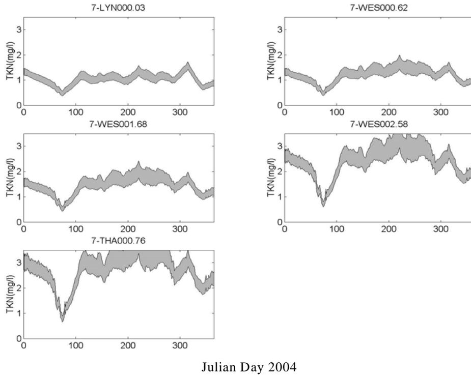
Figure VI.25. Predicted TKN at Western Branch DEQ stations for 2004.
