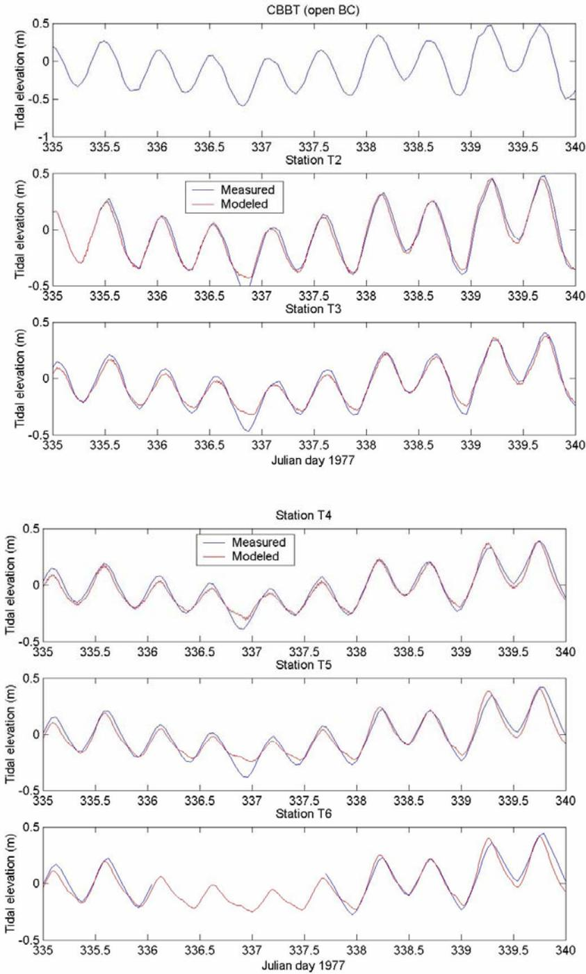
Figure V.6. Real-time comparisons of UnTRIM predictions and NOAA water surface observations.
