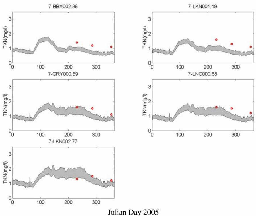
Figure VI.54. Predicted vs. observed TKN at Broad Bay / Linkhorn Bay Branch DEQ stations for 2005.
