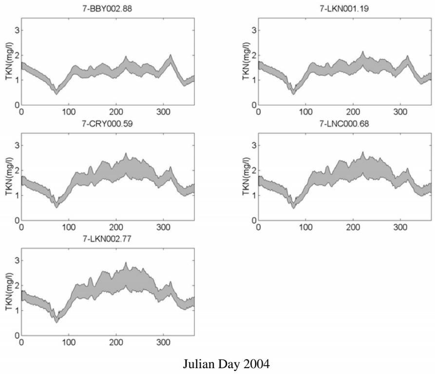
Figure VI.53. Predicted TKN at Broad Bay / Linkhorn Bay Branch DEQ stations for 2004.
