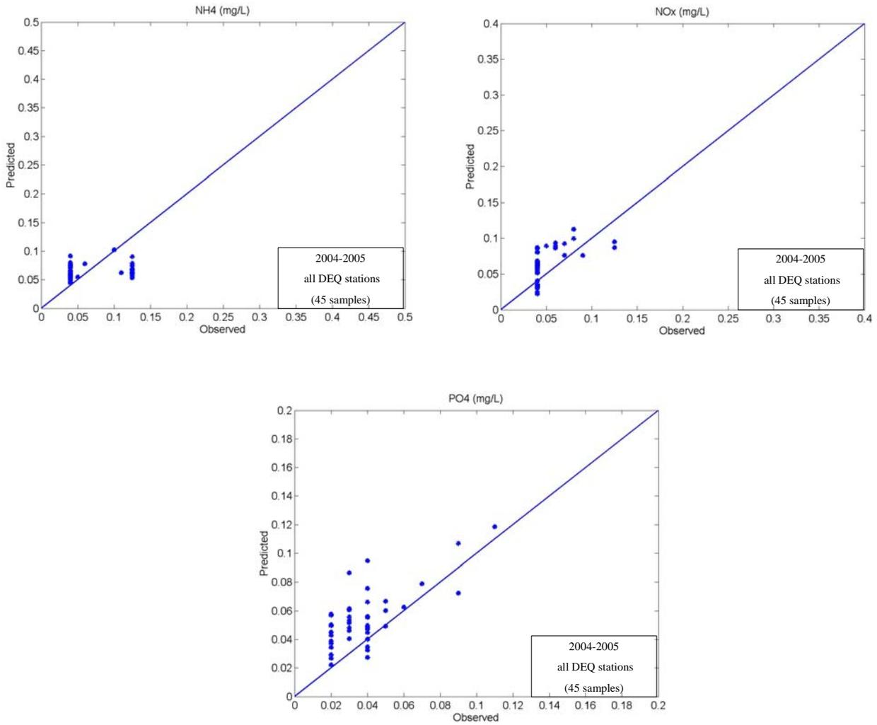
Figure VI.64. Plots of 1:1 predicted vs. observed  $\text{NH}_4$ ,  $\text{NO}_x$ , and DIP TP at all 16 Lynnhaven DEQ stations for 2004 - 2005.
