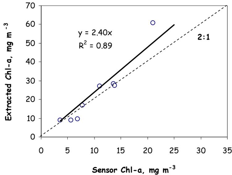
Figure IV.37. Sample calibration plot relating sensor output to measured water quality, in this case chlorophyll-a.
