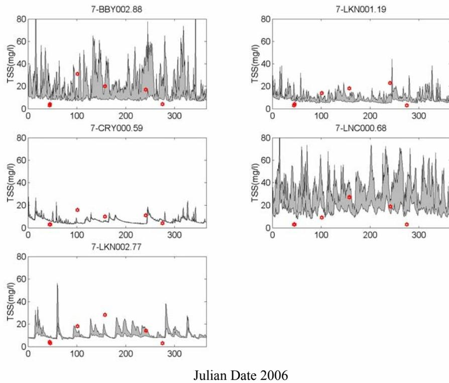
Figure V.44. Predicted vs. observed TSS at Broad Bay / Linkhorn Bay Branch DEQ stations for 2006.
