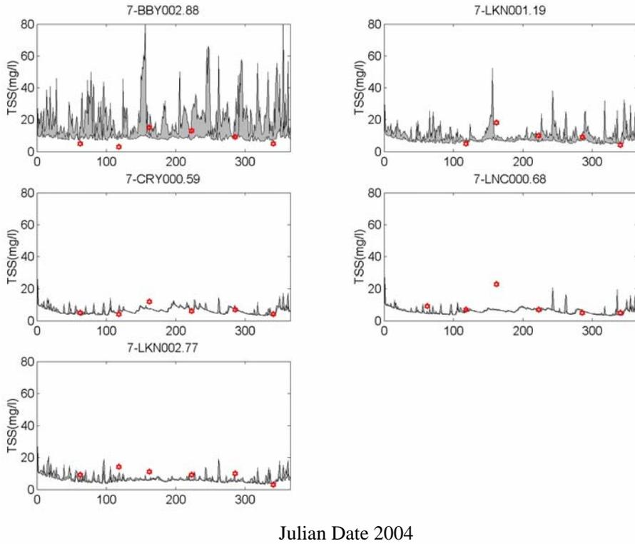
Figure VI.71. Predicted vs. observed TSS at Broad Bay / Linkhorn Bay Branch DEQ stations for 2004.
