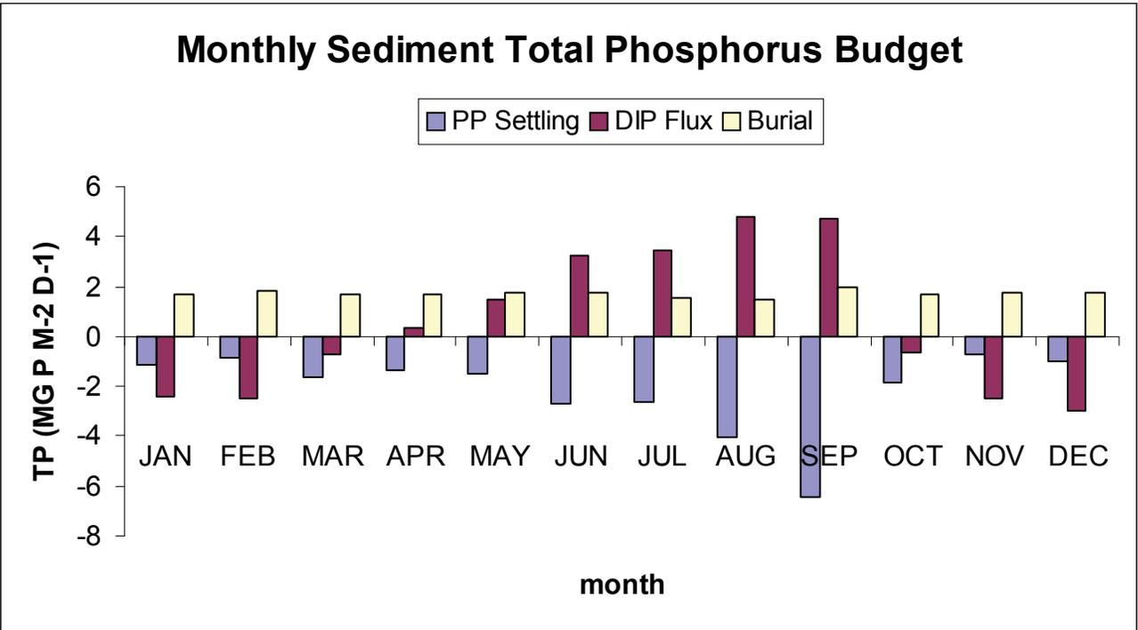
Figure VII.7. Monthly Total Nitrogen budget ( $\text{mg N m}^{-2} \text{d}^{-1}$ ) and Total Phosphorus budget ( $\text{mg P m}^{-2} \text{d}^{-1}$ ) in sediment for Lynnhaven River (positive values indicate leaving sediment, negative values indicate entering sediment)
