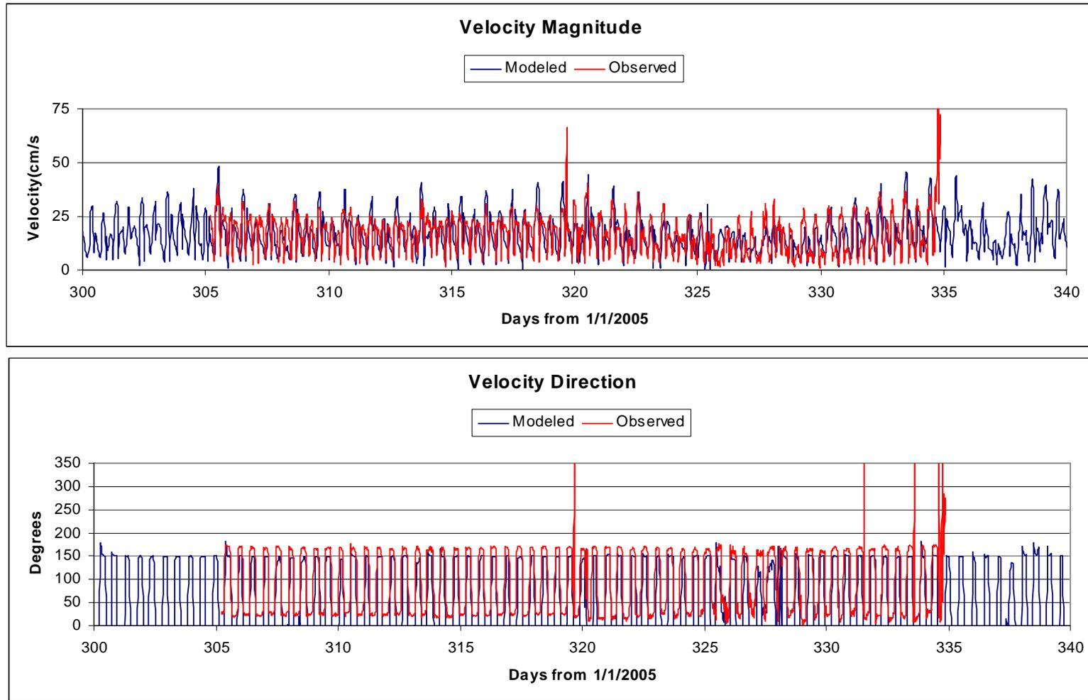
Figure VI.5. Magnitude and direction of measured versus modeled velocity at mid-depth in the Western Branch.
