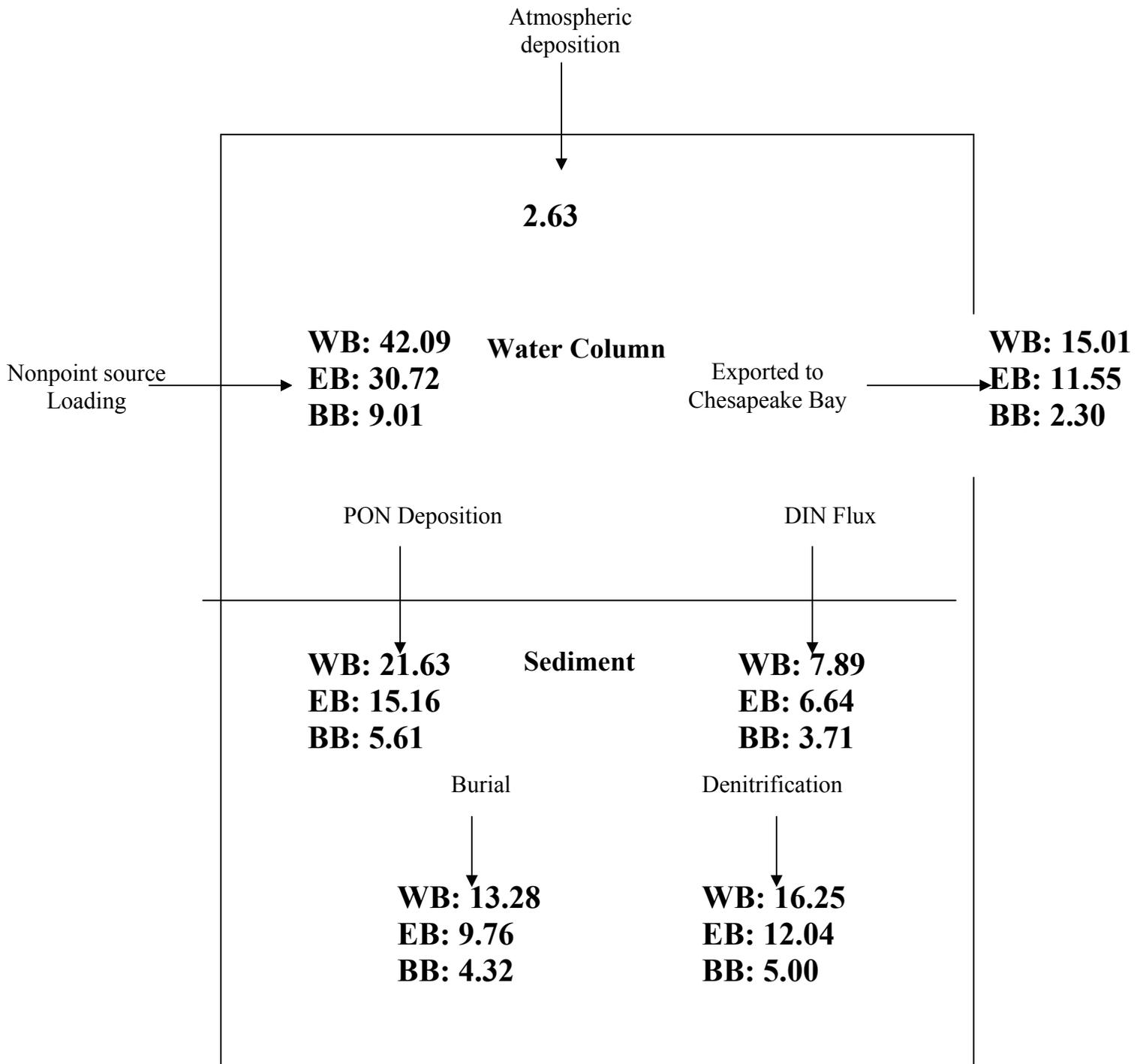
Figure VII.4. Annual Total Nitrogen budget (mg N m<sup>-2</sup> d<sup>-1</sup>) in three branches of Lynnhaven River (WB: Western Branch, EB: Eastern Branch, BB: Broad Bay)
