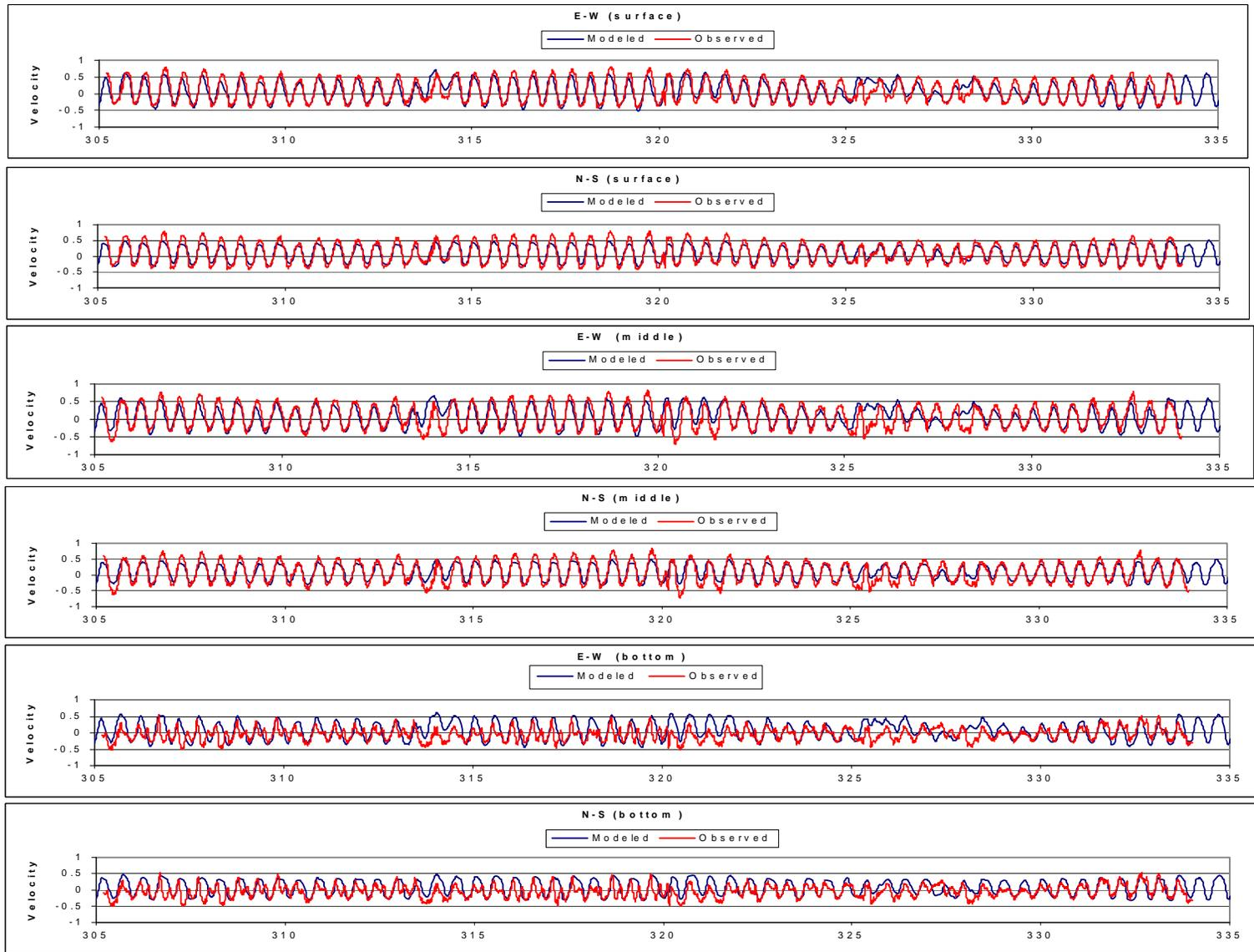
Figure VI.4. East-west and north-south components of measured versus modeled velocity at surface, middle, and bottom layers outside Lynnhaven Inlet.
