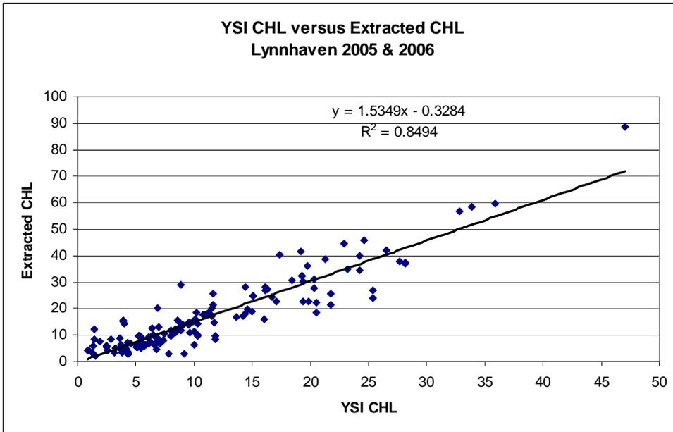
Figure IV.31. 2005-2006 verification station YSI chlorophyll vs. extracted chlorophyll.
