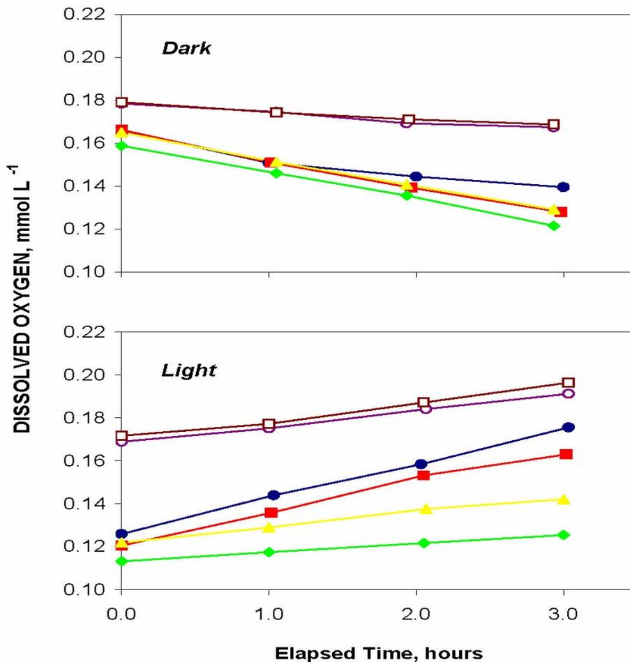
Figure IV.15. Typical time course for DO incubated in the dark and light. Filled symbols depict the sediment cores; open symbols depict the water blanks.
