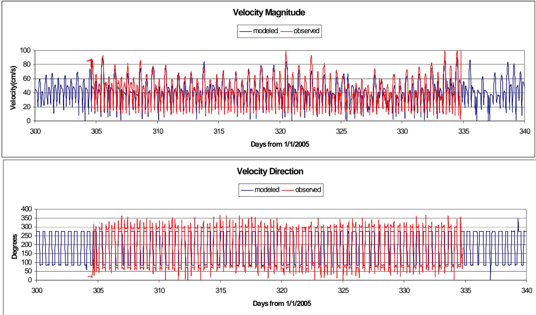
Figure VI.7. Magnitude and direction of measured versus modeled velocity at mid-depth in Broad Bay.
