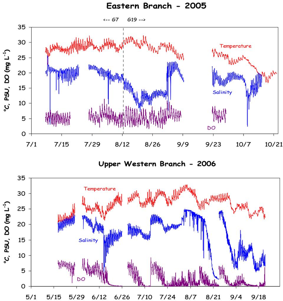
Figure IV.41. Time series measurements of bottom water quality.
