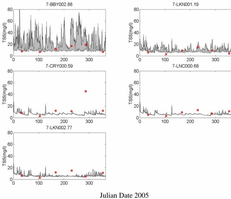
Figure VI.72. Predicted vs. observed TSS at Broad Bay / Linkhorn Bay Branch DEQ stations for 2005.
