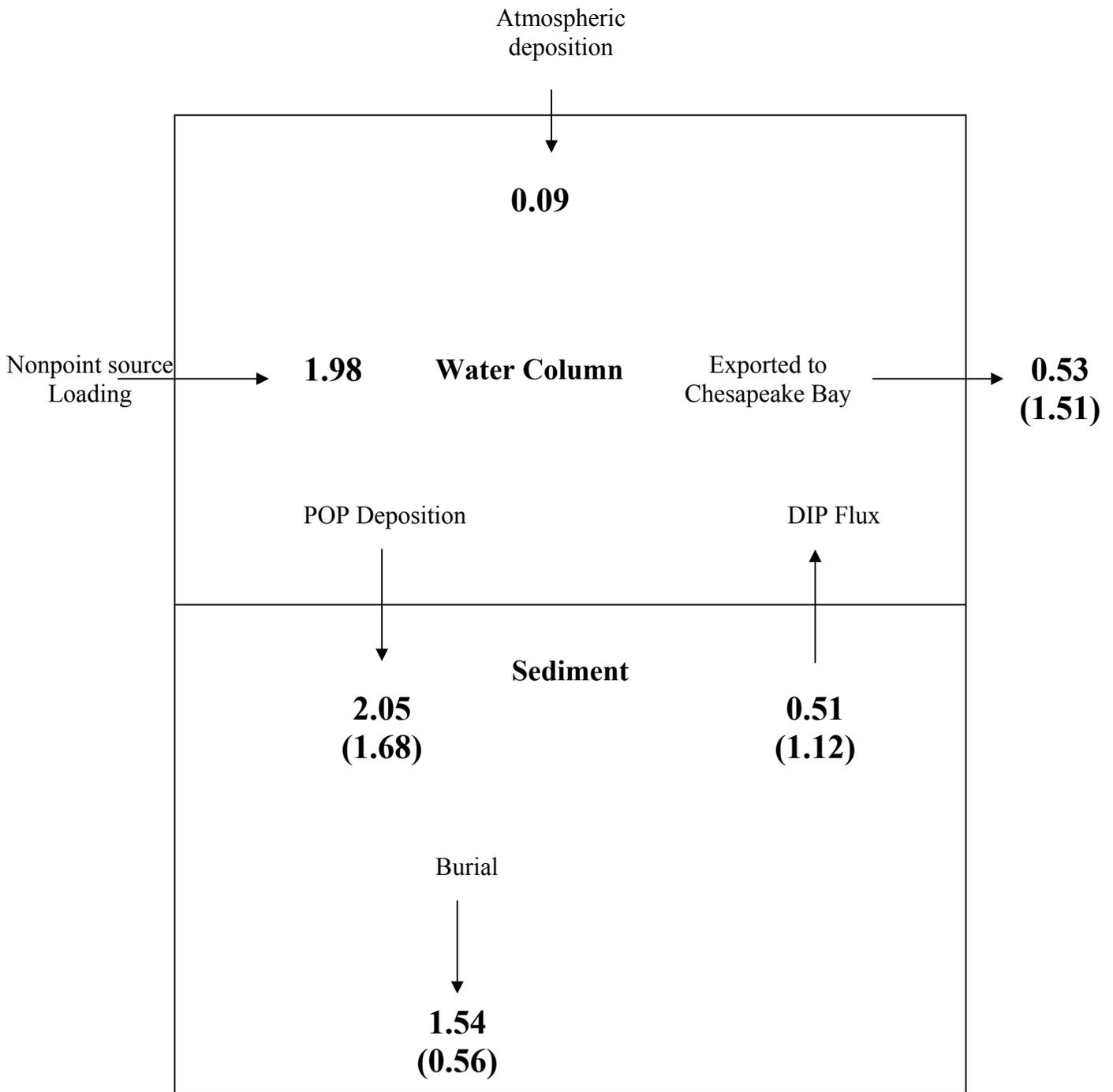
Figure VII.3. Annual Total Phosphorus budget ( $\text{mg P m}^{-2} \text{d}^{-1}$ ) for Lynnhaven River (Values in parentheses indicate results without BMA)
