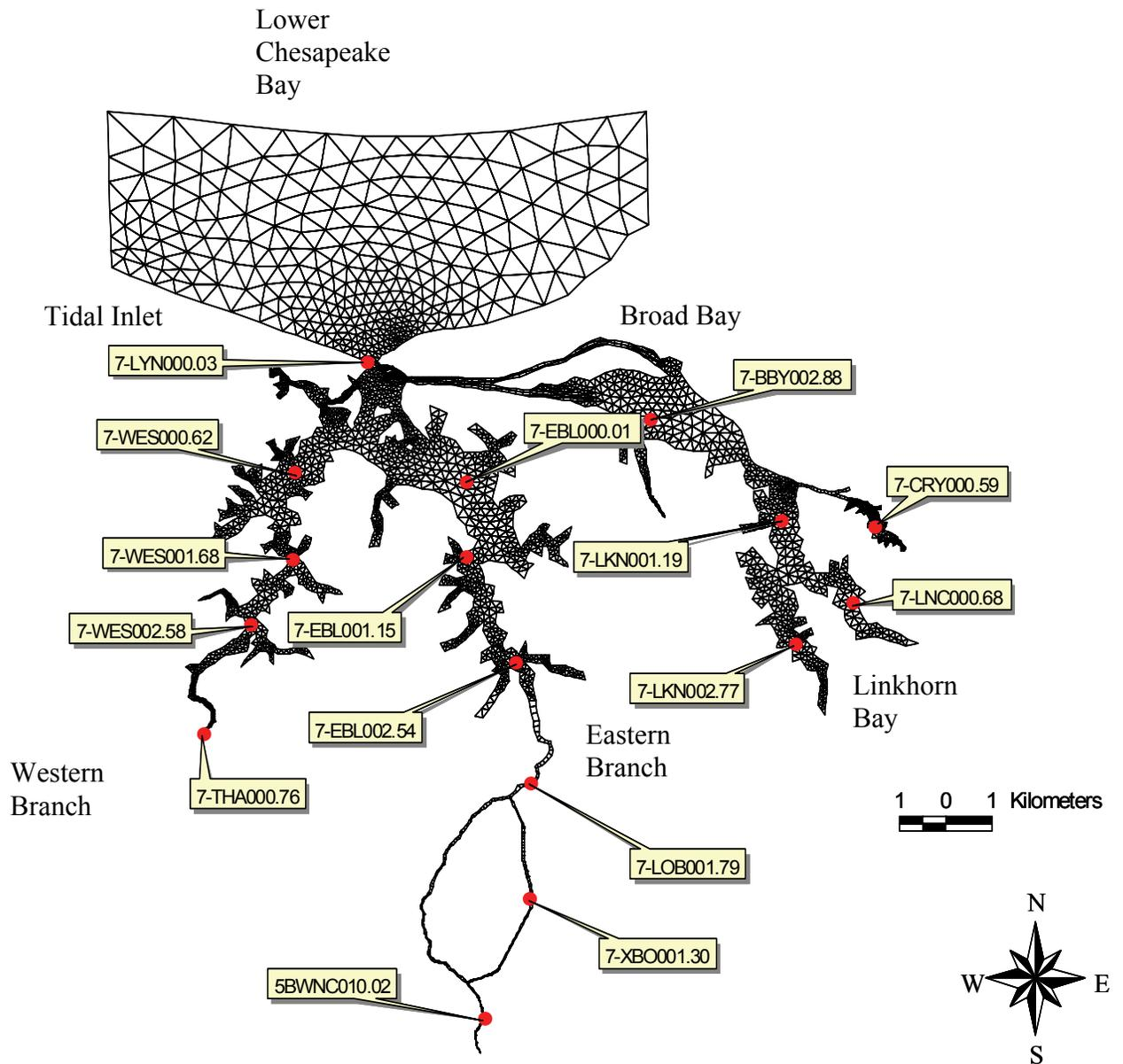
Figure 1. The unstructured grid for Lynnhaven River System and the locations of the 16 Lynnhaven stations monitored by the Virginia Department of Environmental Quality.
