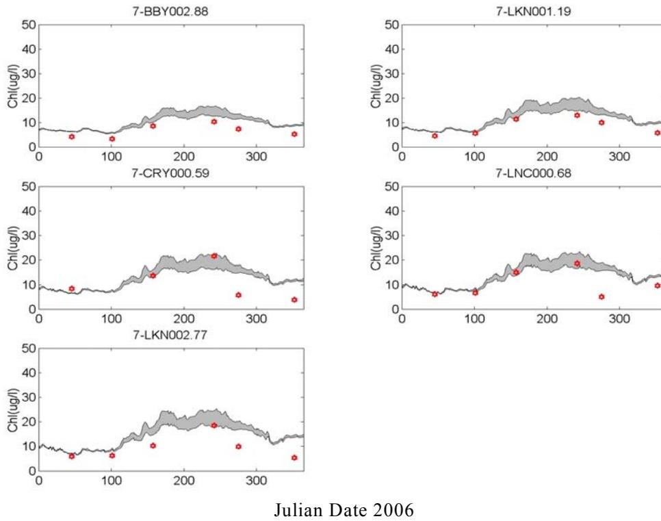
Figure V.34. Predicted vs. observed chlorophyll-a at Broad Bay / Linkhorn Bay Branch DEQ stations for 2006.
