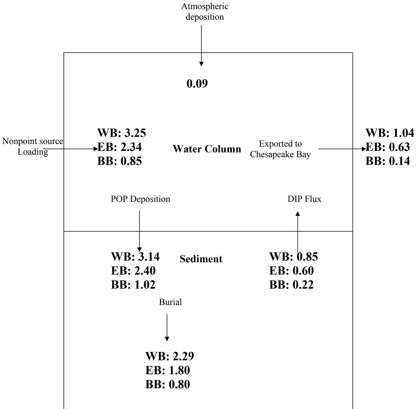
Figure VII.5. Annual Total Phosphorus budget ( $\text{mg P m}^{-2} \text{d}^{-1}$ ) in three branches of Lynnhaven River (WB: Western Branch, EB: Eastern Branch, BB: Broad Bay)
