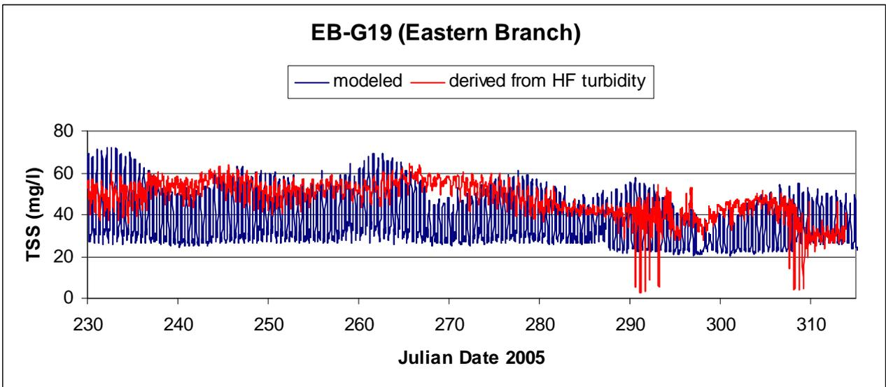
Figure VI.66. Predicted TSS vs. TSS derived from high-frequency turbidity measurements at 3 locations in the Lynnhaven in 2005.
