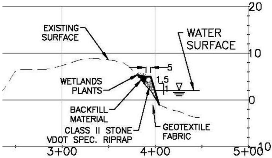
The Lake Windsor (LW) site consists of an eroding fast-land bank ranging from 1 to 3 feet in height. The shoreline is facing south with an effective fetch of about 0.1 miles to the south. The major design features include a trapezoidal stone riprap sill to protect wetland plants and stabilize the shoreline.
