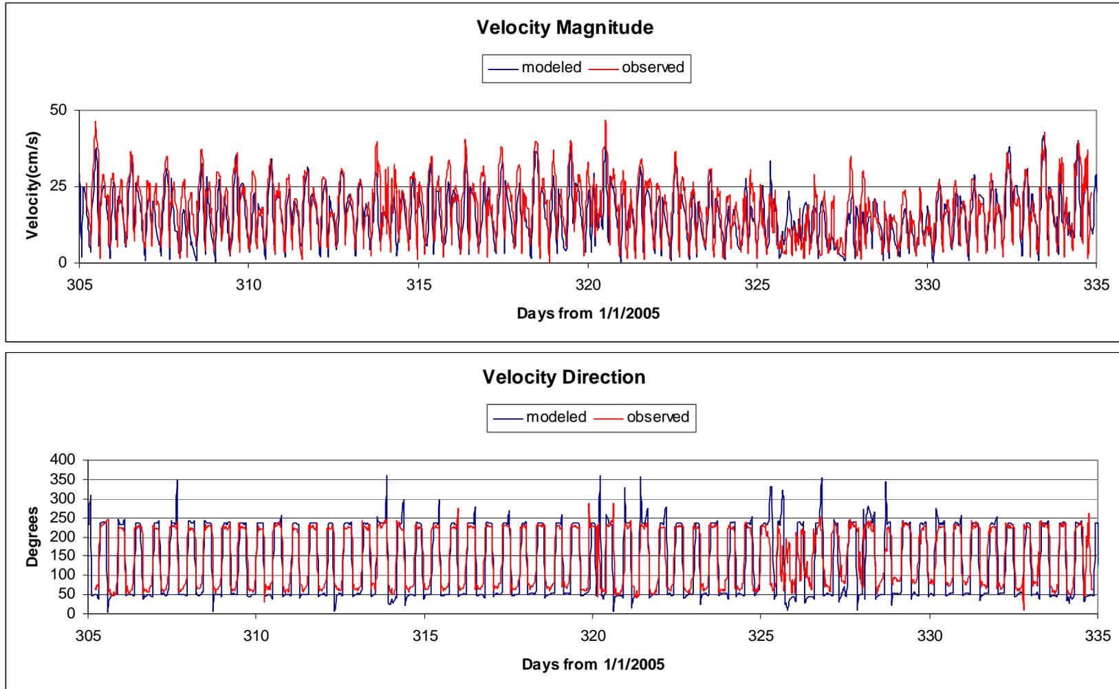
Figure VI.6. Magnitude and direction of measured versus modeled velocity at mid-depth in the Eastern Branch.
