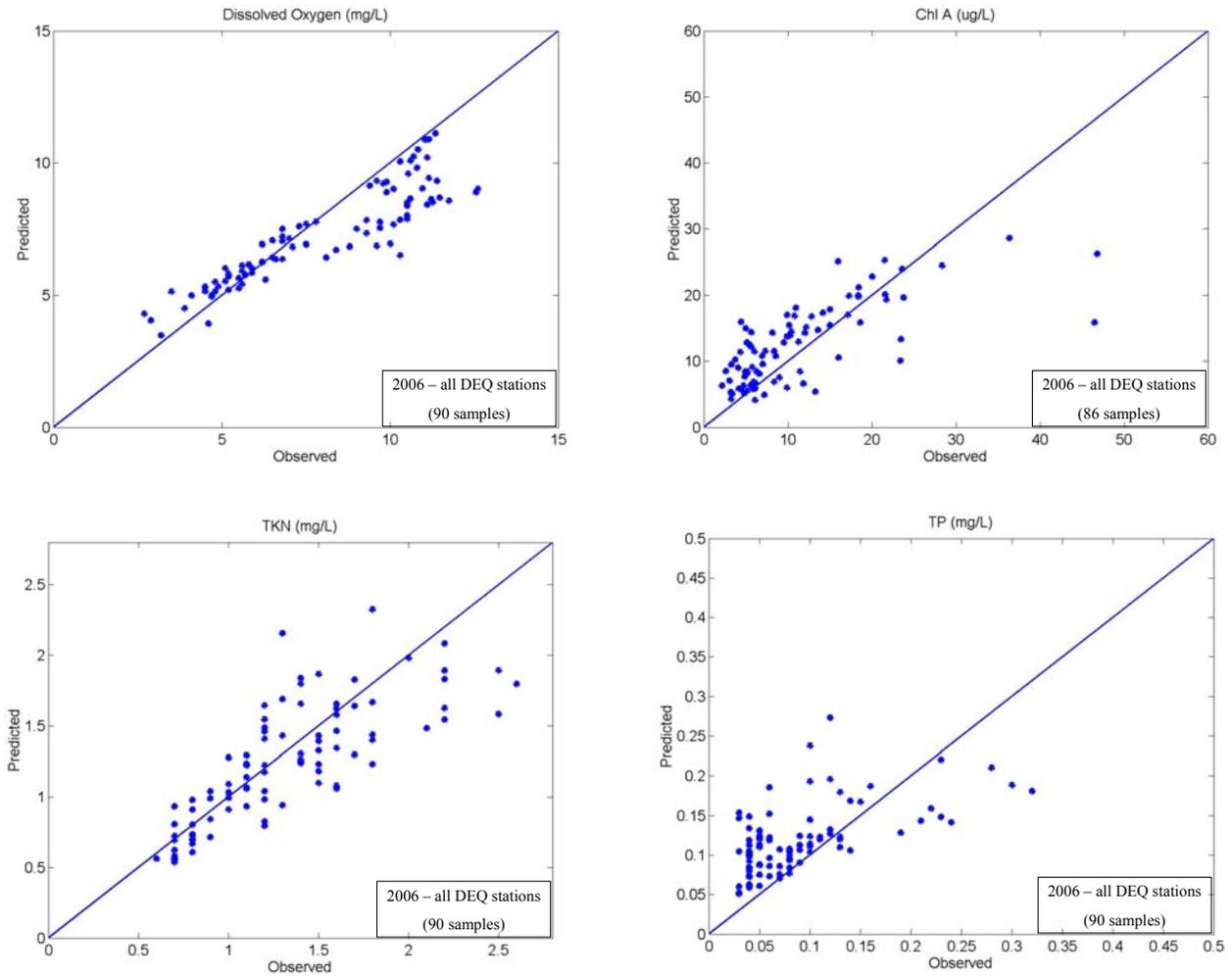
Figure V.40. Plots of 1:1 predicted vs. observed DO, chl-a, TKN, and TP at all 16 Lynnhaven DEQ stations for 2006.
