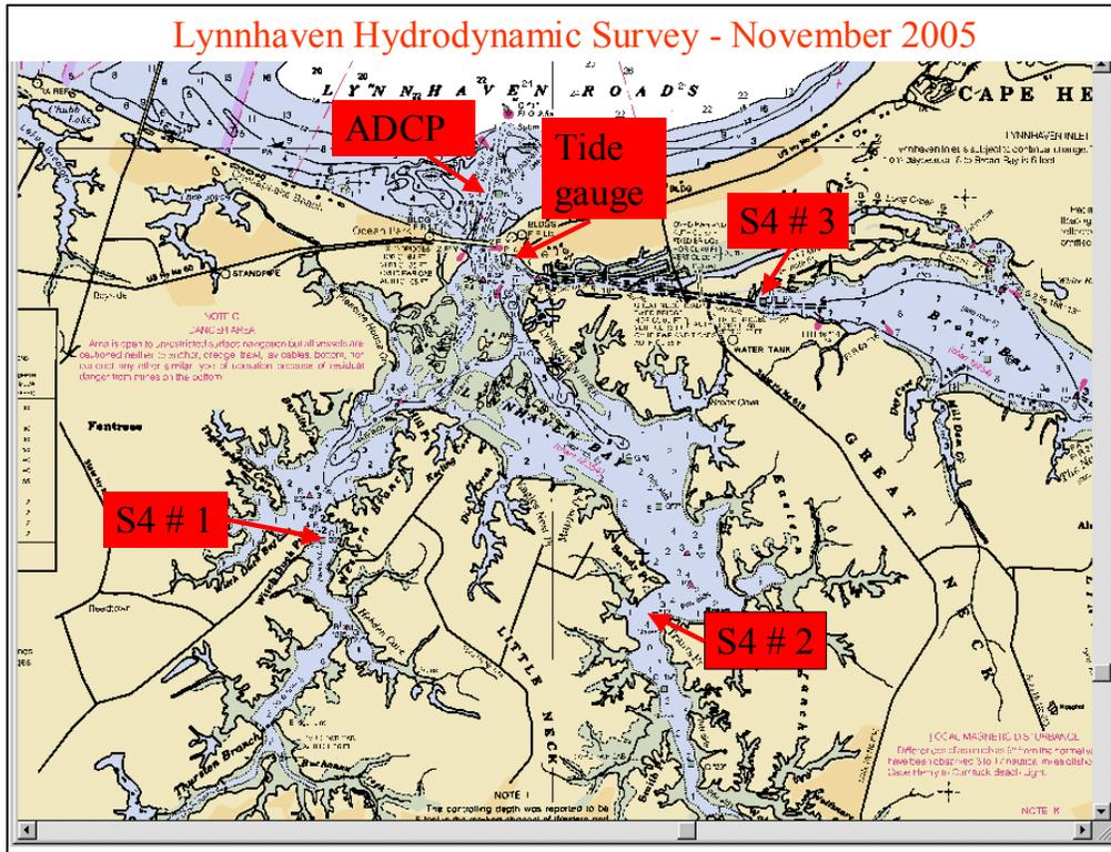
Figure IV.4. Instrument Locations for VIMS Hydrodynamic Survey.
