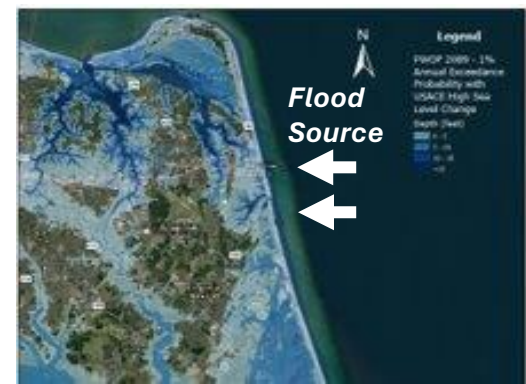
Map: Future Without Project Inundation 1% Annual Exceedance Probability (100yr) at year 2089 with USACE High Sea Level Change
