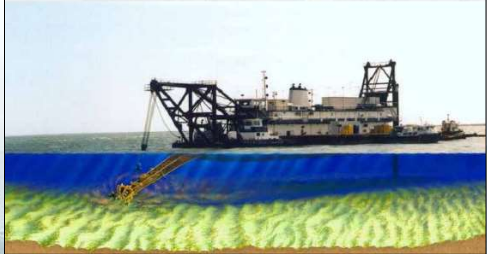
Hydraulic Pipeline / Cutterhead Dredge
