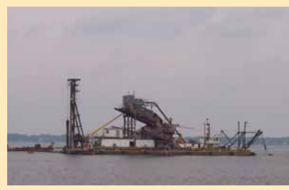
B Dredged material is pumped into one of three active cells
